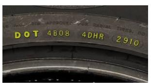
So how can you tell how old your tires are? Stamped into every tire is a four digit date code showing the year and week of manufacture. For example, 2910 means the tire was made in the 29th week of 2010 so it is now 10 years old and should be
